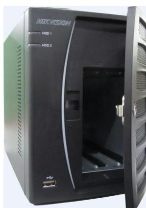
4. Insert the hard disk along the slot until it is placed into position.
