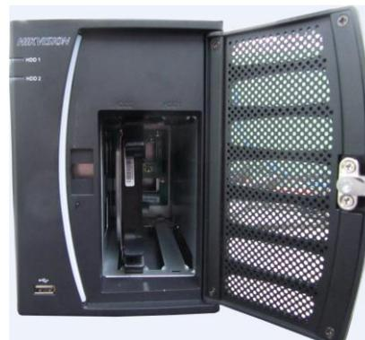
5. Repeat the above steps to install other hard disks onto the NVR. After having finished the installation of all hard disks, close the front panel and lock it with the key again.
